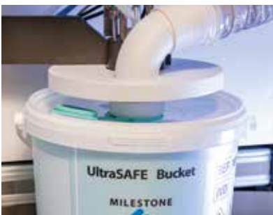
The automatic filling system is lowered and the dispensing nozzle penetrates the seal valve
