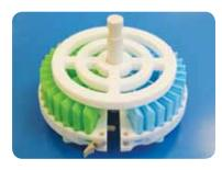
The LOGOS J rack consists of 48 cassettes to allow the flexibility to fit any workload requirements. (Optional: 2 segments of 21 cassettes each)
